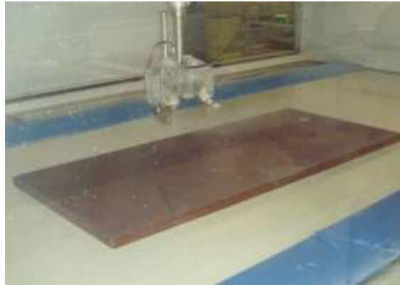
Desktop being sprayed with UV finish
